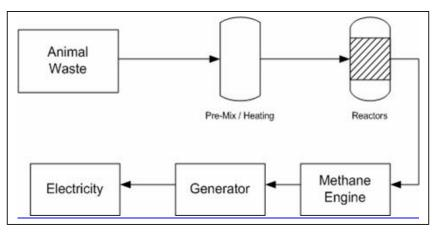
First, the farm waste is feed to pre-mixing tanks where it is heated to  $100 \, ^{\circ}\text{F}$  (38  $^{\circ}\text{C}$ ) which is the optimal temperature for the digestion (or breaking down) of the waste to take place. Next, the feed is sent to reaction tanks where the waste is broken down and gives off biogas. The methane from the reactors is used to power an engine which turns a generator to produce electricity.
