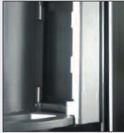
Rotor with hinged metal wiper blades
